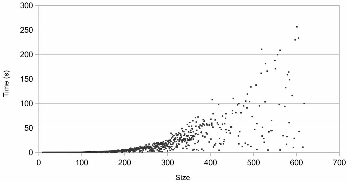
Figure 4: Stress test on randomly generated problems. The  $y$  axis plots the running time in seconds, while the  $x$ -axis is the size  $N$  of the problem, considering the same number  $N$  of activities, pressures and receptors.
